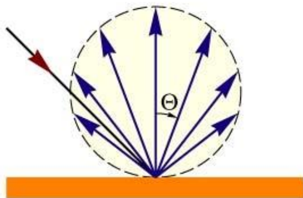
(b) Diffuse (Lambertian) reflector
