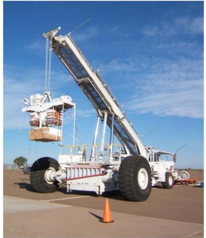
Figure 2. The BalloonSat payload is mounted on the right side of the carrier at the flight line ready for launch. The carrier is suspended from the release vehicle.
