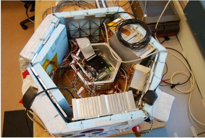
Figure 1. Payload electronics being prepared for launch. Blue foam insulation is placed around the structural walls for thermal control.
