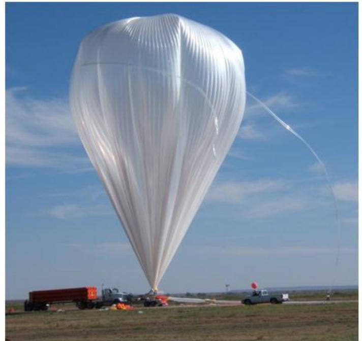
Figure 3. The balloon inflated for launch. Note that this is not the fully inflated volume of the balloon at float altitude.
