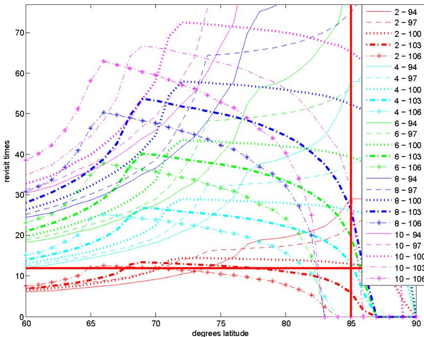
Figure 5. The times per day a latitude is seen by 2-, 4-, 6-, 8-, and 10-satellite Walker delta constellations at 725 km collective altitude, with 94, 97, 100, 103, and 106° collective inclinations, and a sidelooking angle of up to 60 degrees for each satellite. The horizontal red line indicates the minimum revisit times needed to fill the revisit requirement, while the vertical red line indicates the highest latitude (85°) of interest.
