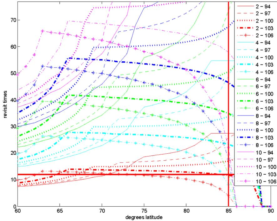
Figure 6. The times per day a latitude is seen by 2-, 4-, 6-, 8-, and 10-satellite Walker delta constellations at 1000 km collective altitude, with 94, 97, 100, 103, and 106° collective inclinations, and a sidelooking angle of up to 60 degrees for each satellite. The horizontal red line indicates the minimum revisit times needed to fill the revisit requirement, while the vertical red line indicates the highest latitude (85°) of interest.
