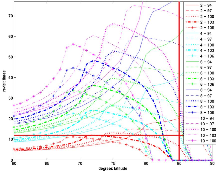
Figure 4. The times per day a latitude is seen by 2-, 4-, 6-, 8-, and 10-satellite Walker delta constellations at 450 km collective altitude, with 94, 97, 100, 103, and 106° collective inclinations, and a sidelooking angle of up to 60 degrees for each satellite. The horizontal red line indicates the minimum revisit times needed to fill the revisit requirement, while the vertical red line indicates the highest latitude (85°) of interest.
