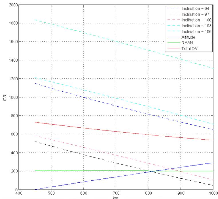
Figure 7. Total  $\Delta V$  for an altitude change to a 450 km orbit from an initial circular orbit of 500 to 1000 km, an inclination change from SSO to 94, 97, 100, 103, and 106 degrees, with the total  $\Delta V$  calculated for change to 97 degrees, and a RAAN change of  $1^\circ$ .
