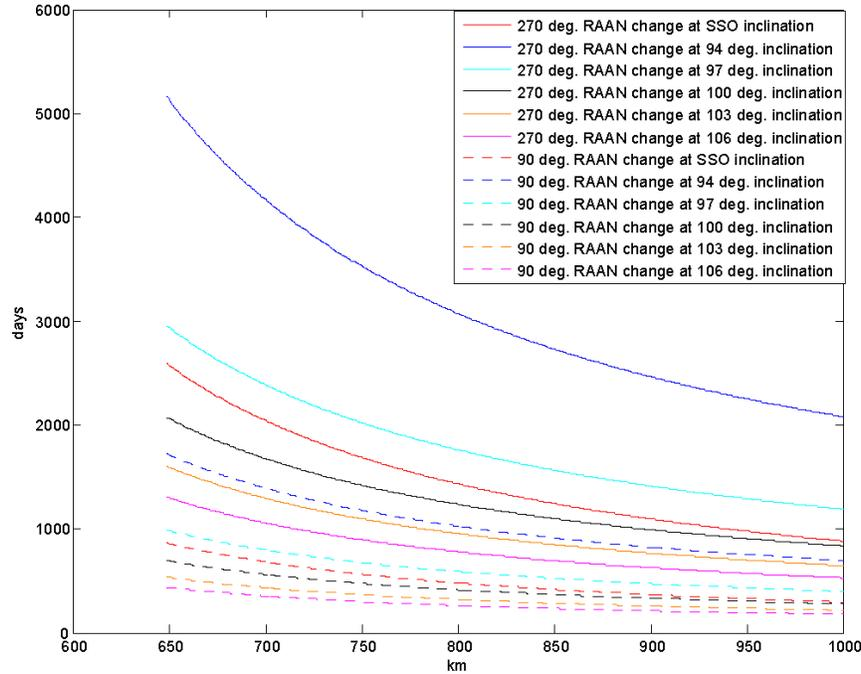
Figure 10. Days taken for the last and first satellite in Figure 9 to precess from an initial circular orbit ranging from 650 to 1000 km altitude (any lower initial orbits would have started to take a prohibitively long time). The cases of RAAN precession up to 270° and 90°, with 94, 97, 100, 103, and 106 inclination and initial orbit SSO inclinations for all satellites, is presented.
