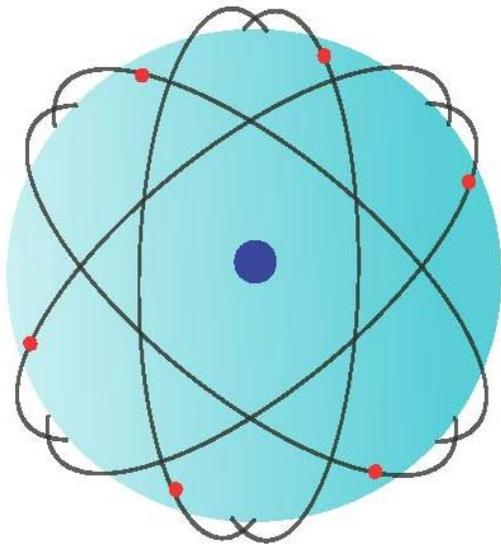
Figure 3. As an example, a pole-view of the rosette-like Walker delta 6-satellite configuration. The red dots represent satellites.
